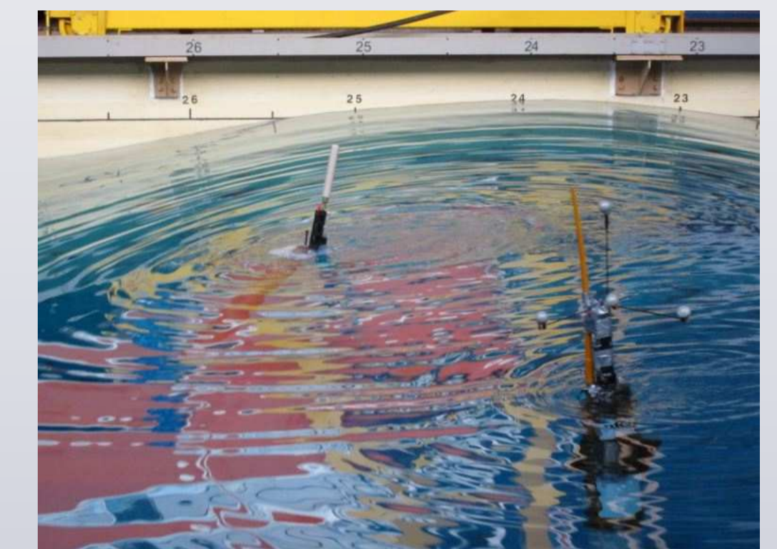
Swell testing in pool
