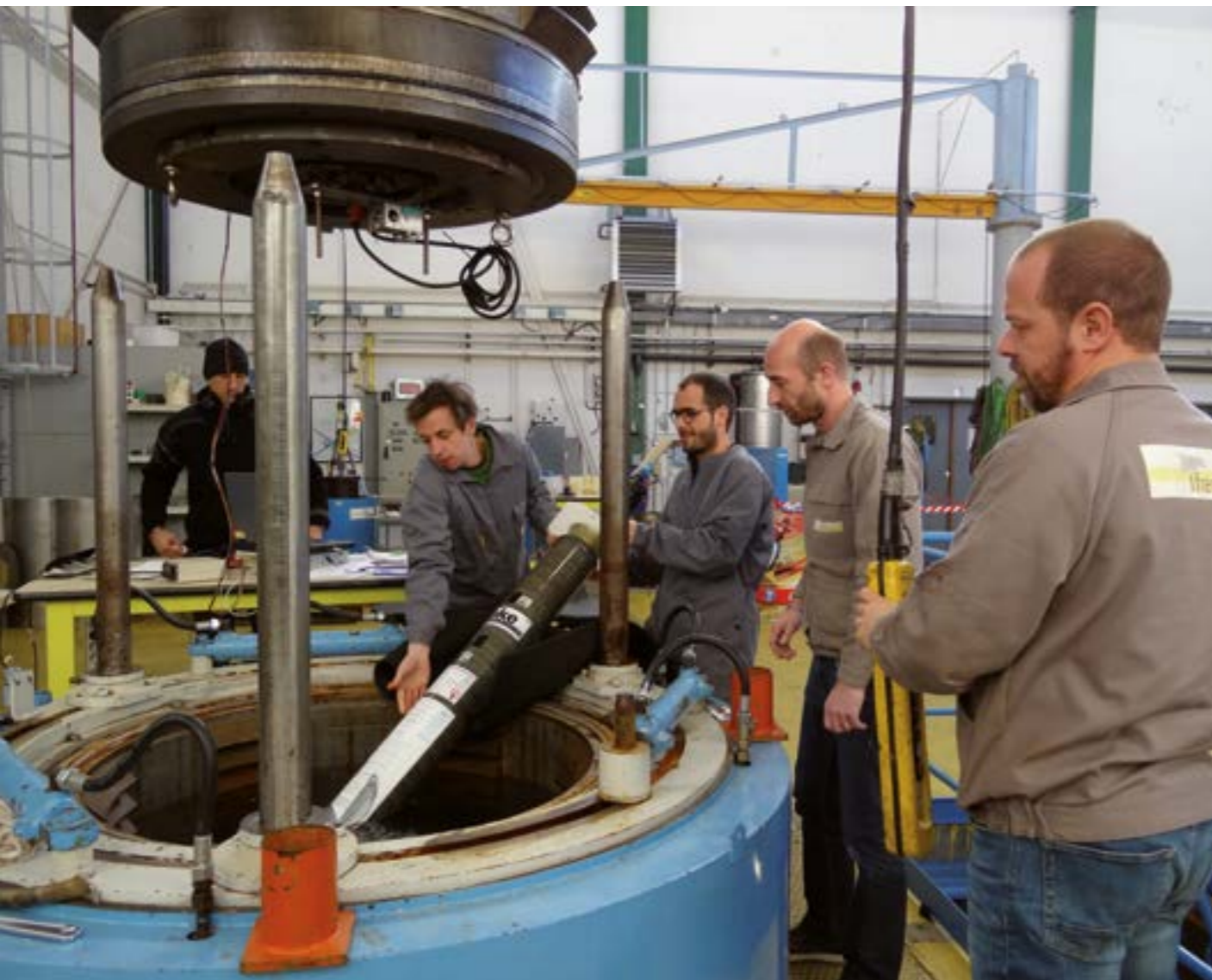
A Deep Argo float tested at the hyperbaric chamber of Ifremer facility, to reproduce the extremely high pressures of the abyssal zone.
