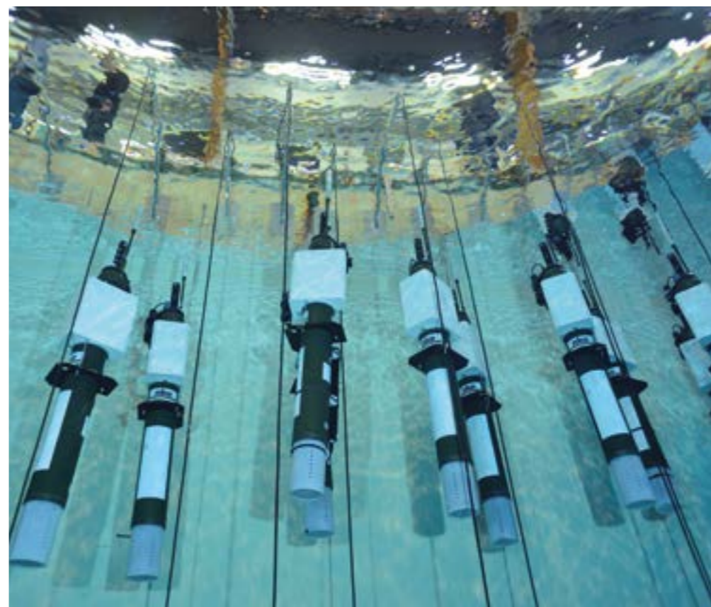
Biogeochemical Argo floats tested at the Ifremer facility.
