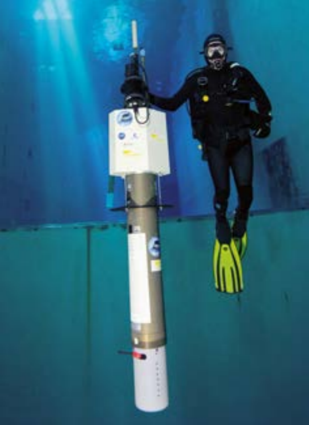
A BGC float at the Ifremer facility, in the unique 20-metre depth pool tank where Argo floats are tested.
