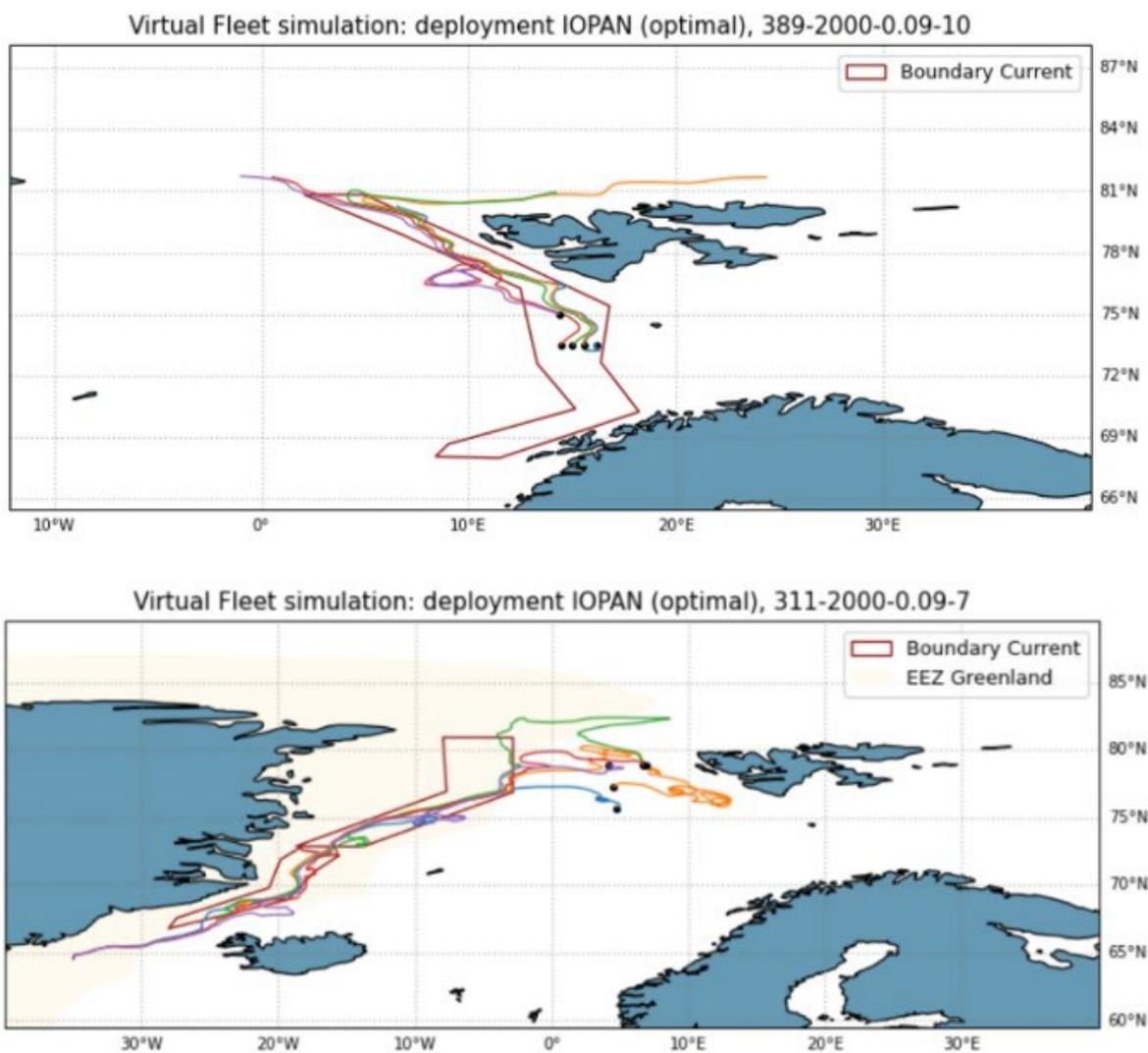
Figure 9. Simulations of the best trajectories using the optimum deployment positions from the AREX cruises and the optimum mission configurations in the WSC (top) and ECG (bottom)
