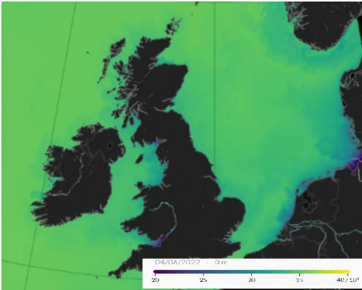
Figure 11. Salinity field based on the CMEMS Ocean Physics Analysis and Forecast product of the Atlantic - European North West Shelf region. For the production of the model's output Argo profiles have been utilised (<https://doi.org/10.48670/moi-00054>)
