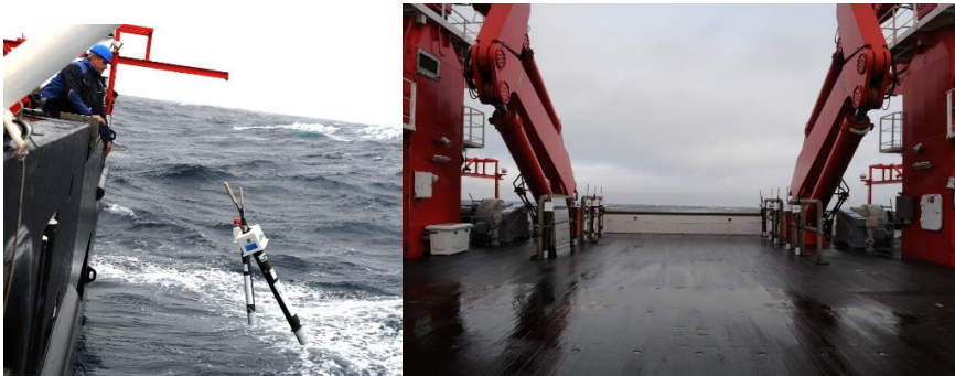
Fig.3: Deployment of Arvor floats equipped with RBR and SBE CTDs in January 2021 on RV Sonne cruise SO280.
