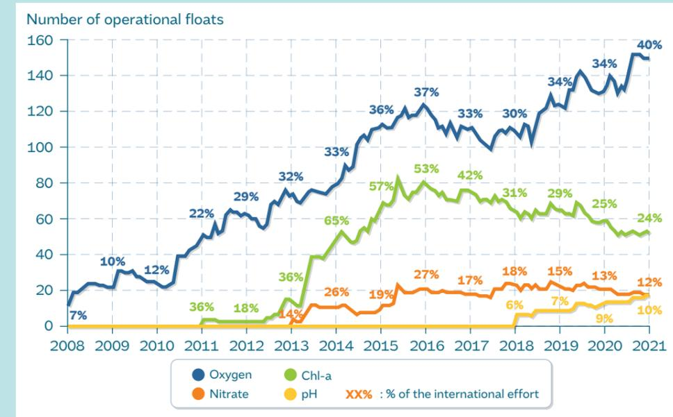
Figure 10: Evolution of the European contribution to four of the six biogeochemical parameters, in number of active Euro-Argo floats measuring that variable (left axis, solid curve), and percentage of active Euro-Argo floats measuring that variable in the global array (percentage of each year on the curves). © OceanOPS/AIC
