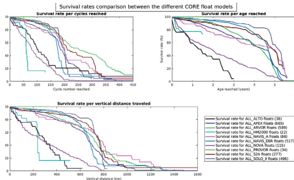
Figure 5 : CORE float models survival rates comparison
