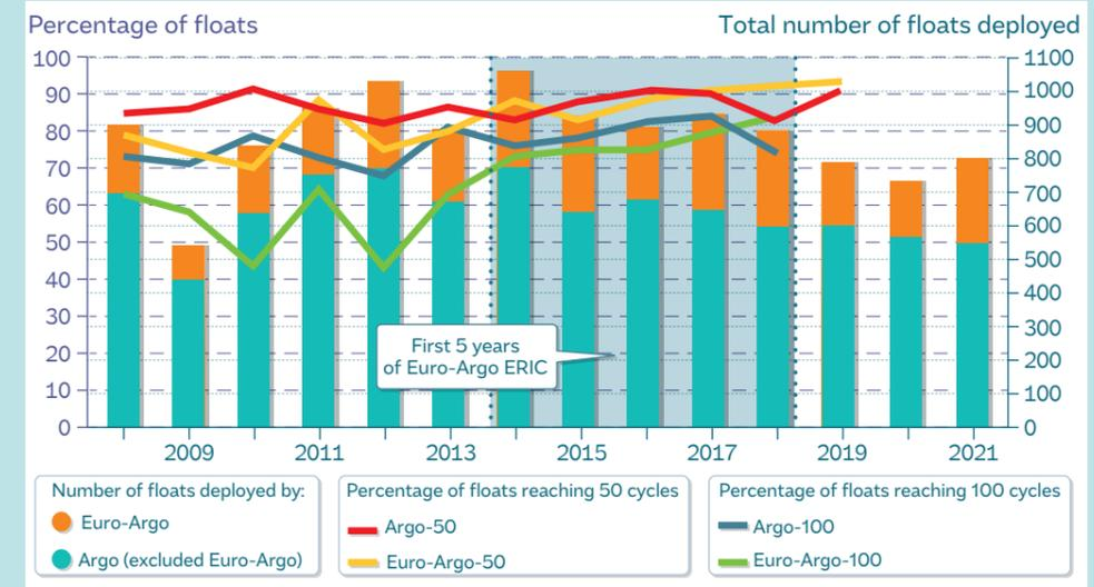
Figure 11: Percentage of floats reaching the 50 or 100 cycles target compared to the Argo fleet (coloured lines, left axis) and total number of floats deployed (right axis). Since 2015, the performance of the Euro-Argo fleet has steadily improved both in reliability (50 cycles) and longevity (150 cycles target). © OceanOPS/AIC
