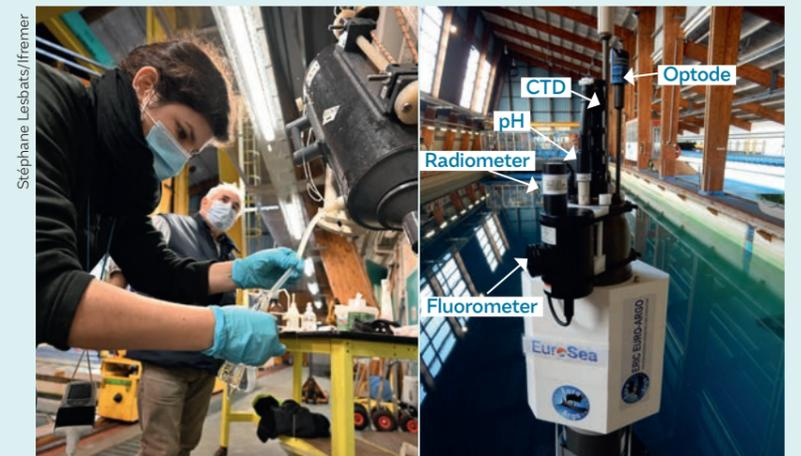
Acceptance tests of the BGC floats in February. Left: Water samples collected and further analysed by Ifremer/LOPS. Right: EuroSea NKE PROVOR CTS4 float with its BGC sensors.
