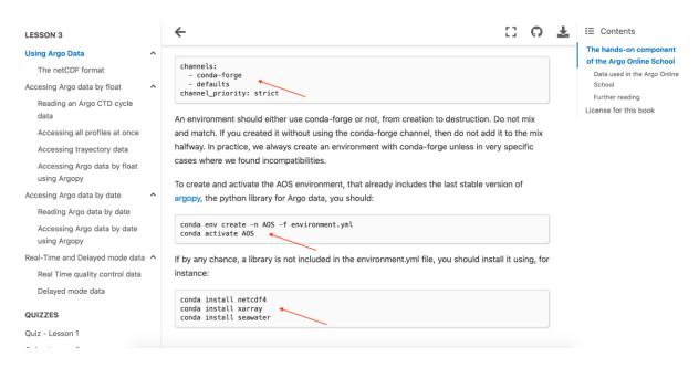
Fig 3. AOS set up for the hand-ons component in lesson 3.
