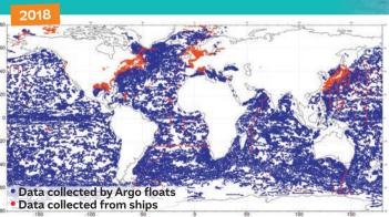
Positions of measurement points (temperature, pressure and salinity profiles) collected with research vessels or Argo floats.
