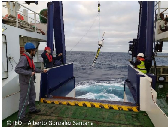
Figure 7: Arvor-I/RBR float deployment on the morning of Dec. 11 st 2020.
