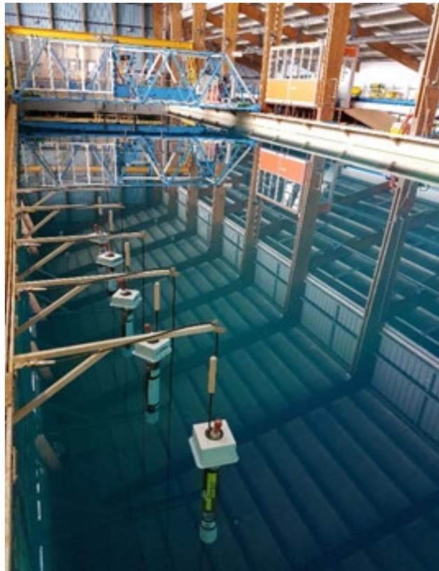
Figure 4: Qualification with 5 Arvor-I RBR in the seawater tank at IFREMER
