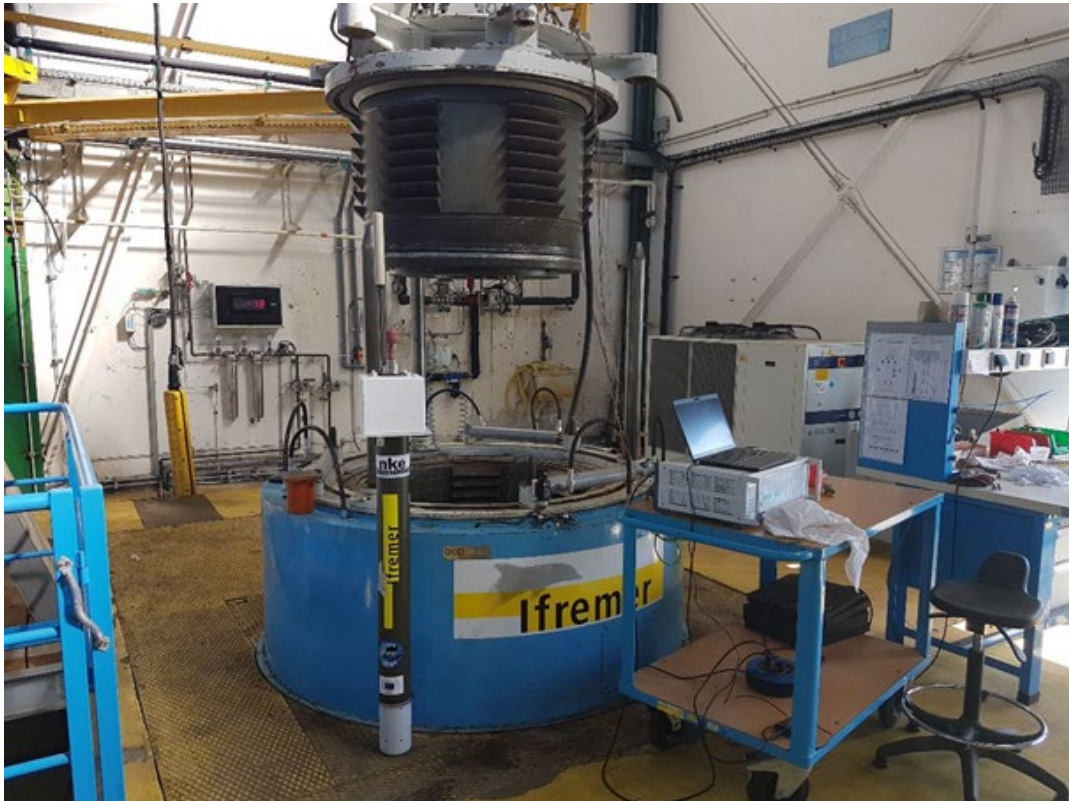
Figure 5: Qualification of an Arvor-I RBR in hyperbaric tank at IFREMER
