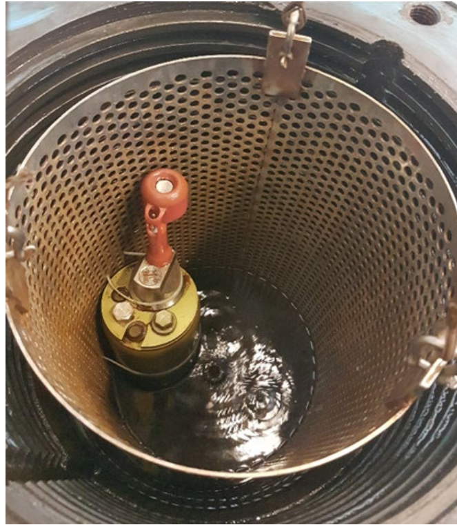
Figure 3: Qualification of the Arvor-I RBR adaptor part
