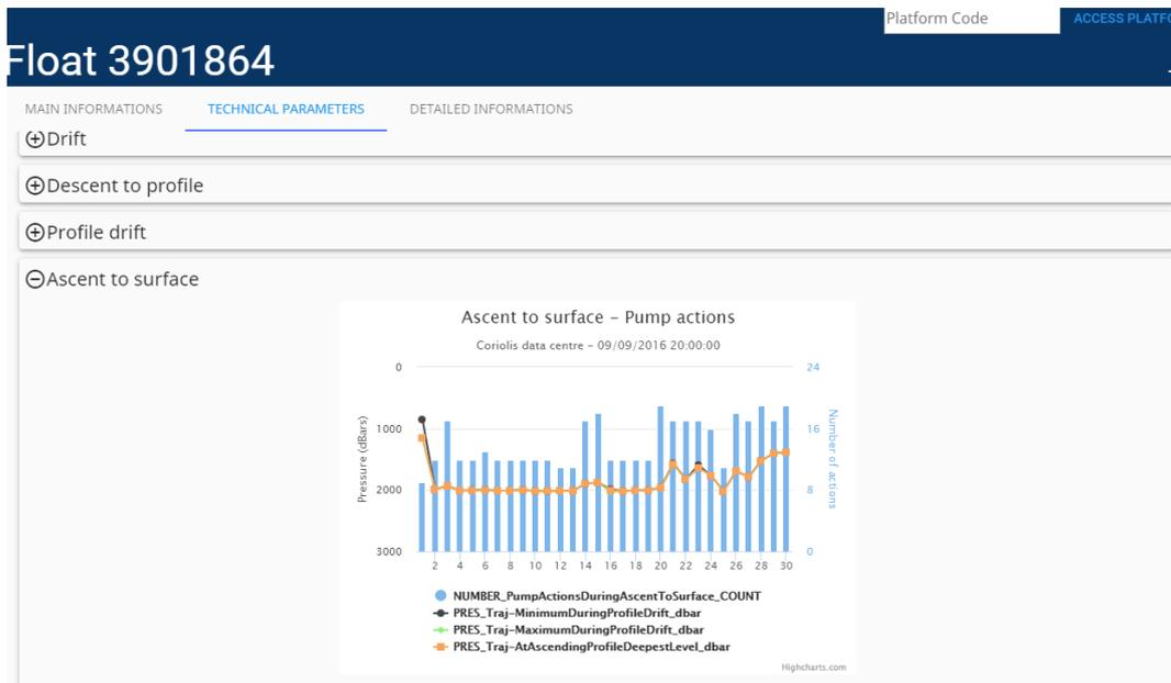
Figure 16: Float webpage – technical parameters tab with Ascent to surface graph unfolded
