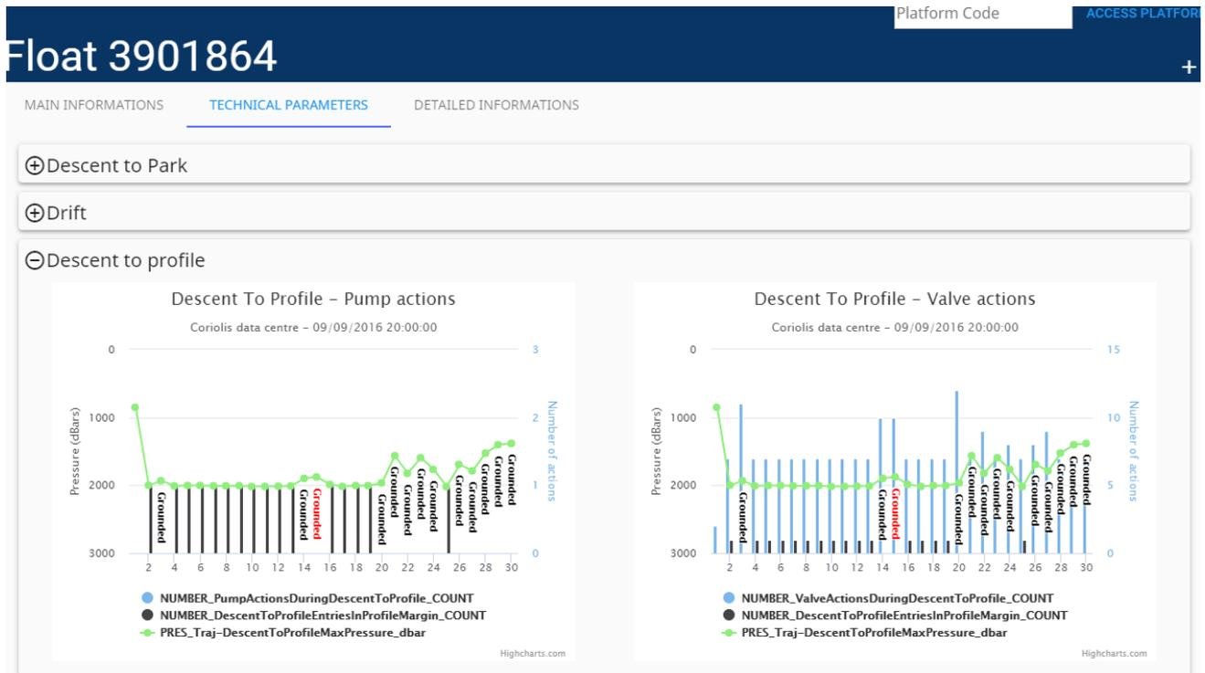
Figure 14: Float webpage – technical parameters tab with Descent to Profile graphs unfolded.
