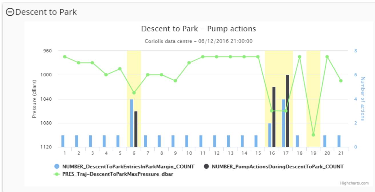
Figure 34: FLAG\_DescentToPark\_TooFast\_LOGICAL, FLAG\_DescentToPark\_StabilizationProblem\_LOGICAL and FLAG\_DescentToPark\_MaxPressureAnomaly\_LOGICAL alerts.
