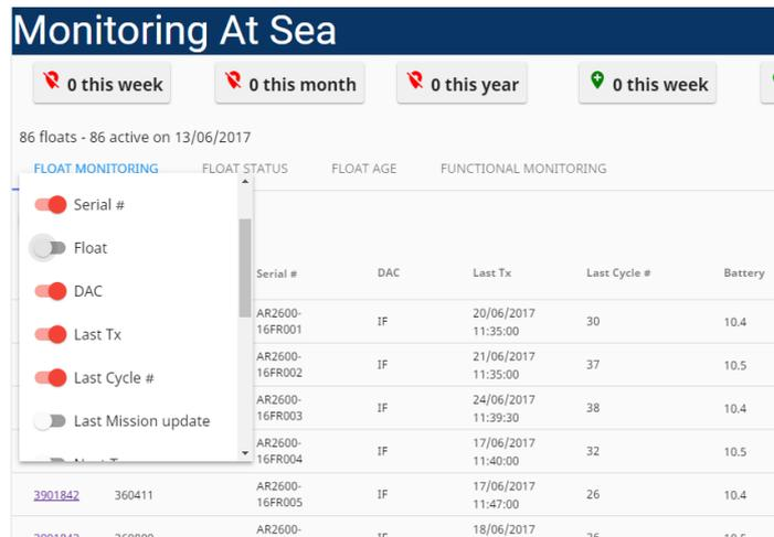
Figure 22: Fleet dashboard – listing: selection of column fields
