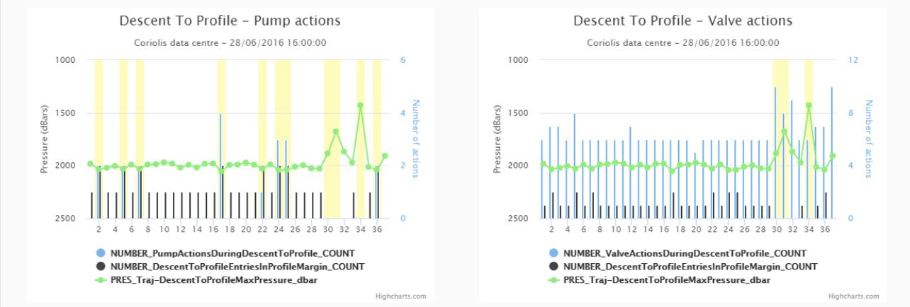
Figure 36: FLAG\_DescentToProfile\_TooFast\_LOGICAL and FLAG\_ProfileMaxPressureAnomaly\_LOGICAL alerts.
