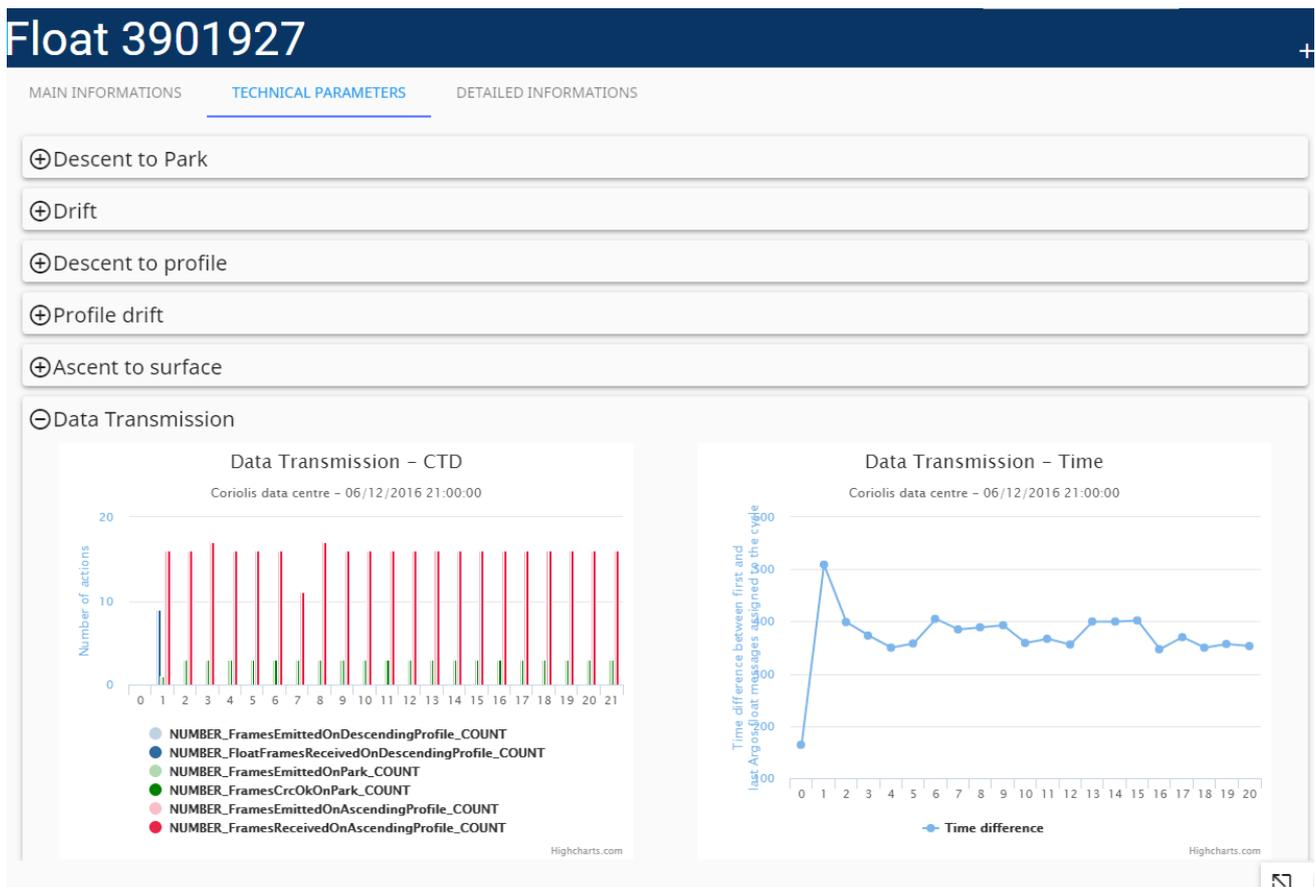
Figure 18: Float webpage – technical parameters tab for data transmission. Example for a MOCCA Argos transmission with the comparison between emitted and received frames (left) for different measuring phases. The transmission time on surface for each cycle is also monitored (right).
