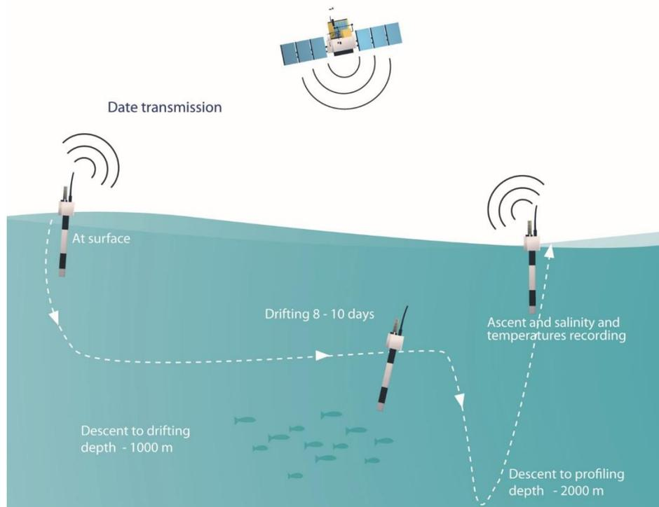
*Figure 11: Standard Argo mission cycle phases.*
