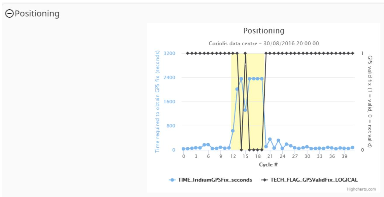
Figure 20: Float webpage– technical parameters tab for GPS positioning.
