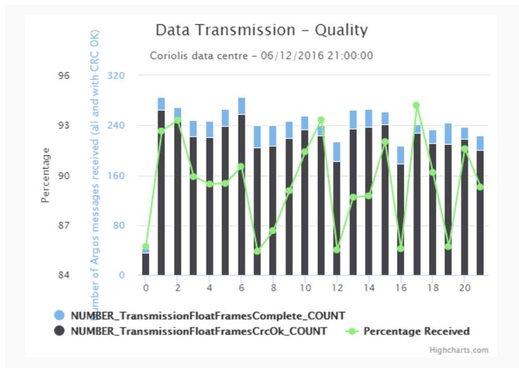
Figure 19: Float webpage – technical parameters tab for data transmission. Example for a MOCCA Argos transmission with the ratio between the number of received messages and the number of received messages that have a good CRC.
