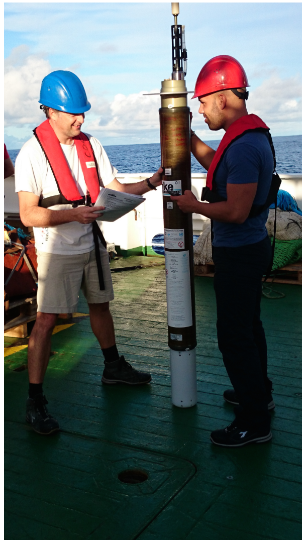
Figure 2. Argo's configuration step through Bluetooth connection before the deployment phase.
