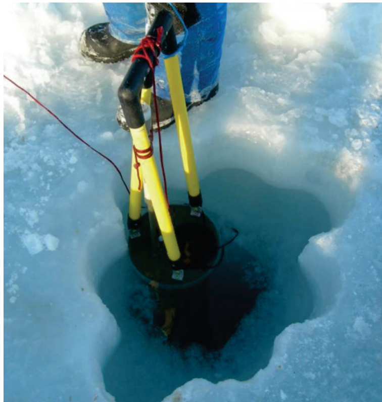
Figure 10. The firm ice bumper applied by the NKE in a modified PROVOR float. Credit: NKE
