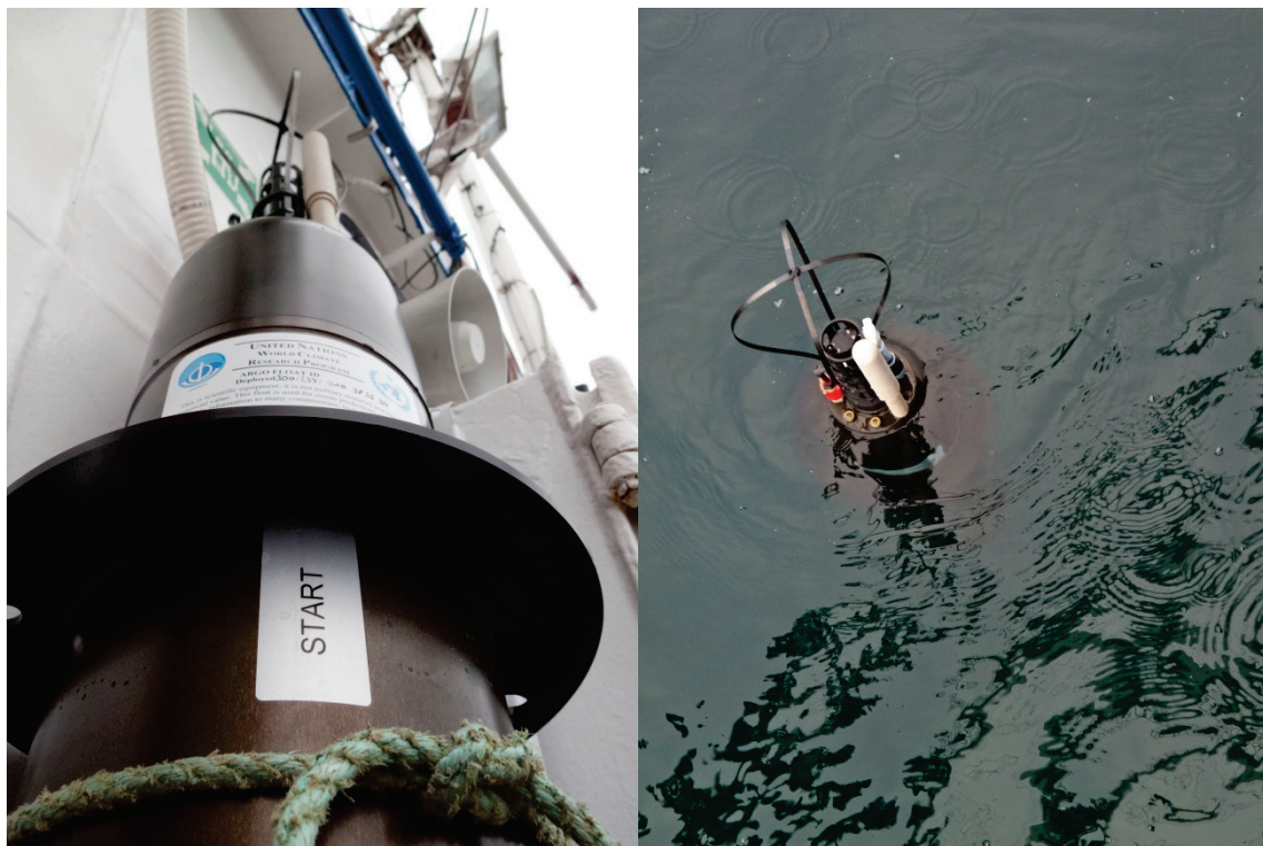
Figure 12. The NEMO float with INS mounted internally deployed in the West Spitsbergen Current in summer 2014 (photo I. Goszczko, IOPAN)
