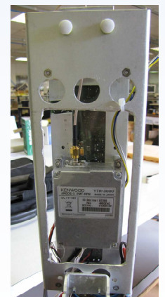
Integration of the Argos-3 transmitter on Arvor profiling floats
