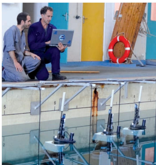
Figure 26: Testing phase of AtlantOS floats (pictured: Biogeochemical) by the Euro-Argo technical team in the Ifremer tank during summer 2017.
